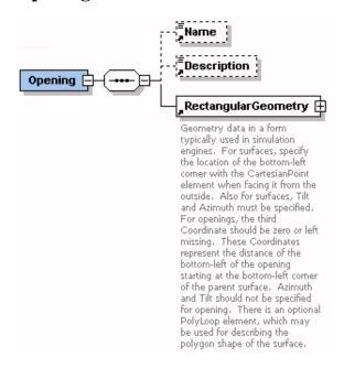
This element is used by TRACE® 700 to define glass areas within a wall or roof surface.
