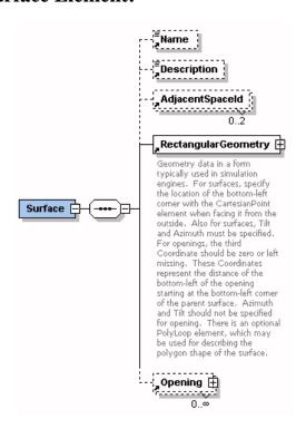
TRACE® 700 imports wall, roofs, partitions, and exposed floors from the surface element.
